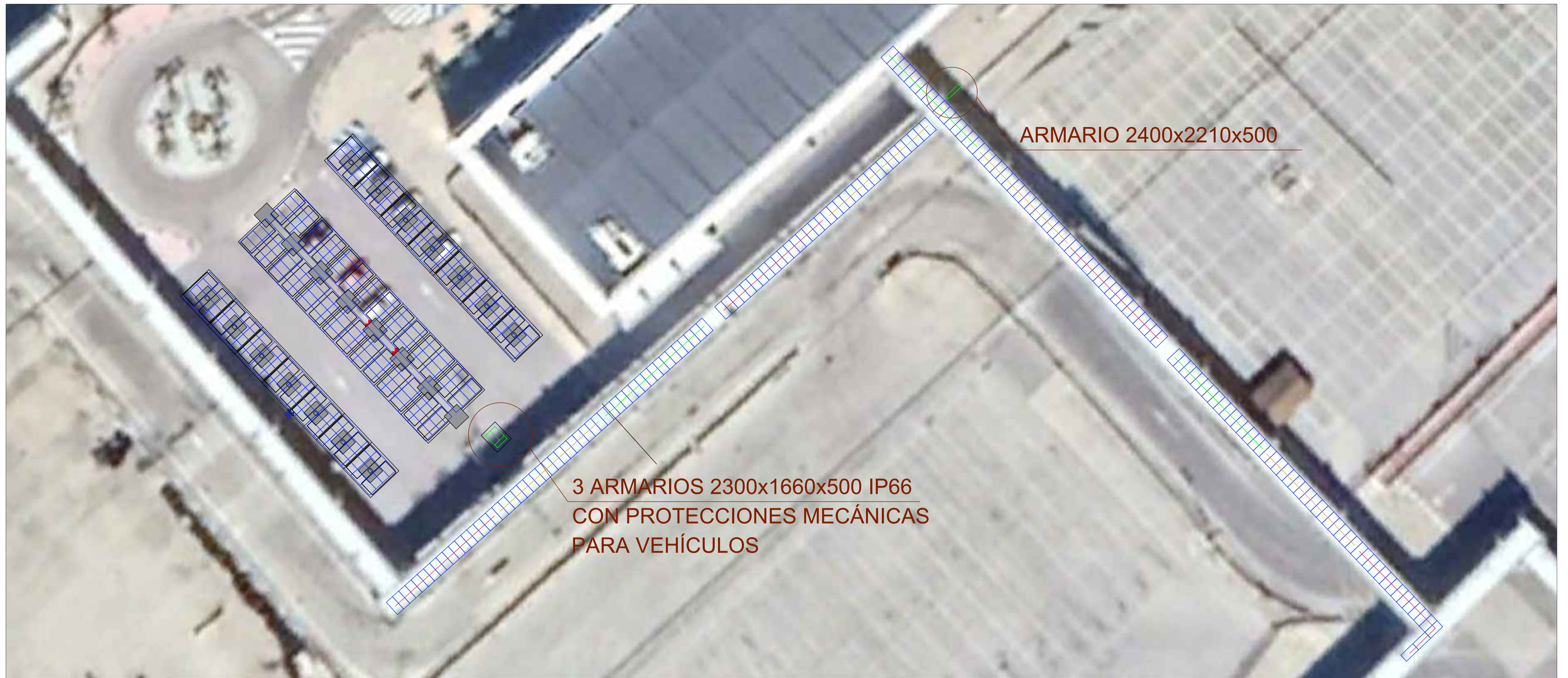
ARMARIO INVERSORES 40 kW 2400X2210X500 IP66
