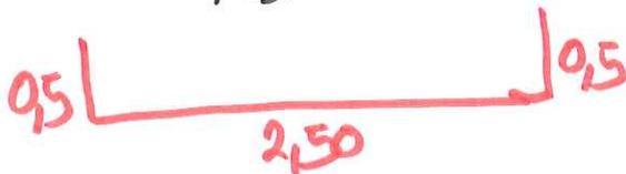
$$\begin{aligned} \text{Kg ACERO} &= 18 \times 2 \times 2,47 \times 3,5 = \\ &= 312 \text{ Kg} \rightarrow 67 \text{ Kg}/\text{m}^2 \end{aligned}$$
